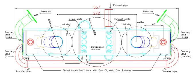
Bore: 80mm, Stroke: 100mm(50+50)
