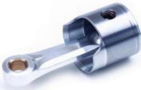
A beefy, machined-aluminum conrod connects the piston to the crank. The piston includes an oil groove for lubrication and a modified piston skirt for better air/fuel flow through the boost port.
