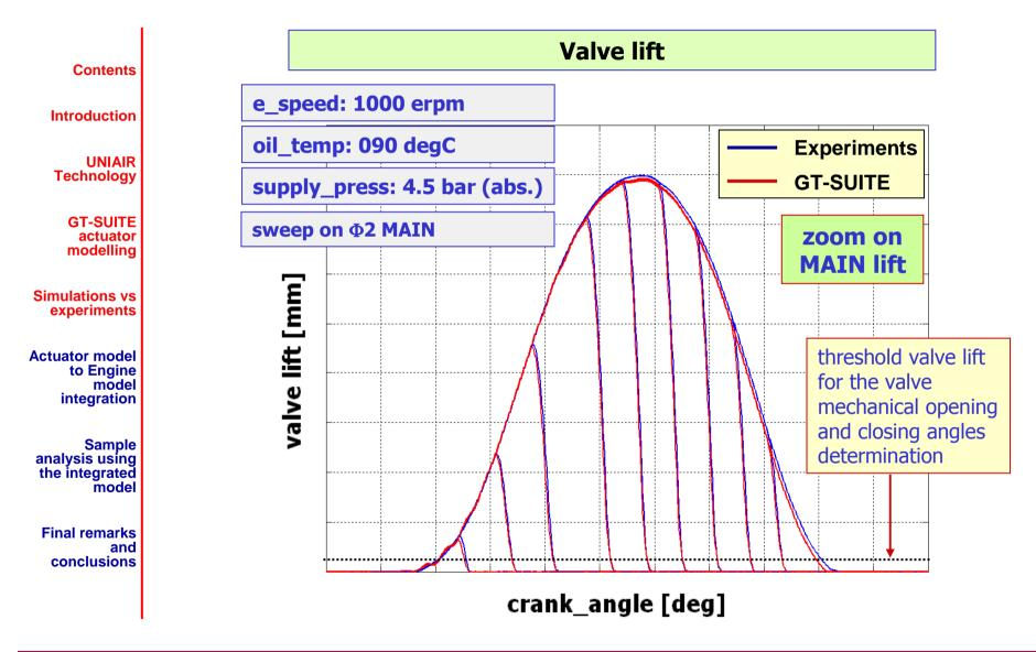
Comparison between simulation results and experimental data Actuator characteristic maps - valve closing angle vs SV control
