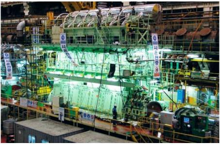
Fig. 2 – Wärtsilä 7RT-flex82C on test bed.
